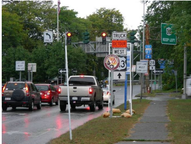
Sign density and arrangement is confusing
